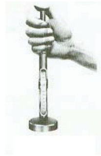
Gambar 10.3 Mesin uji kekerasan Shore scleroscope. c. Type PHS-3
