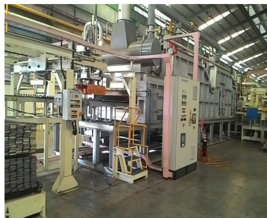
Gambar 2.5 Heating furnace Plant 3b PT. Indospring Tbk
