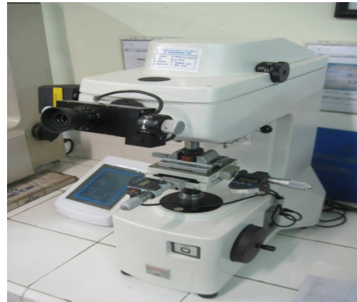
Gambar 2.21 Mikro Vickers , Type HM, Mitutoyo
