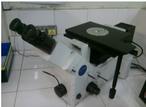
Gambar 2.22 Struktur mikro scope, Type GX 51, Olympus
