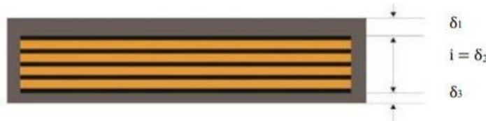
Gambar 4. Penampang belt conveyor
